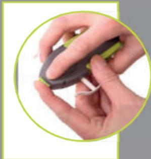
The last measured width value is stored in the device. To call it up, **press the front measuring tongue fully in and switch on the instrument at the same time**. You can then carry out the shoe measurement directly (Attention: Check length adjustment.)
