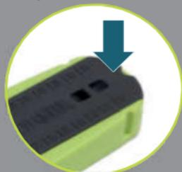
**After three beeps**, the measurement is complete. Remove the meter from the shoe and read the result on the display. **The result is displayed for 40 seconds**, and then you will hear five short beeps to signify the end of the measuring process and the display flashes again. Now you can make another measurement by inserting the meter into another shoe.
