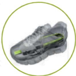
**The inside shoe measurement is carried out automatically while the measuring device sits inside the shoe for at least 6 seconds.**
