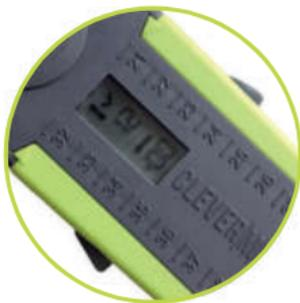
*The lower display shows the remaining space in width(mm).*
