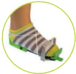
To **measure the foot width**, press the width clamps together to the side of the child's foot, and then additionally press in the front measuring tongue until you hear two beeps. The foot width is now saved.
